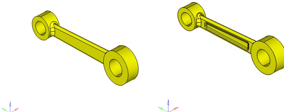
Figure 4: Original and Optimized Model of Connecting Rod
