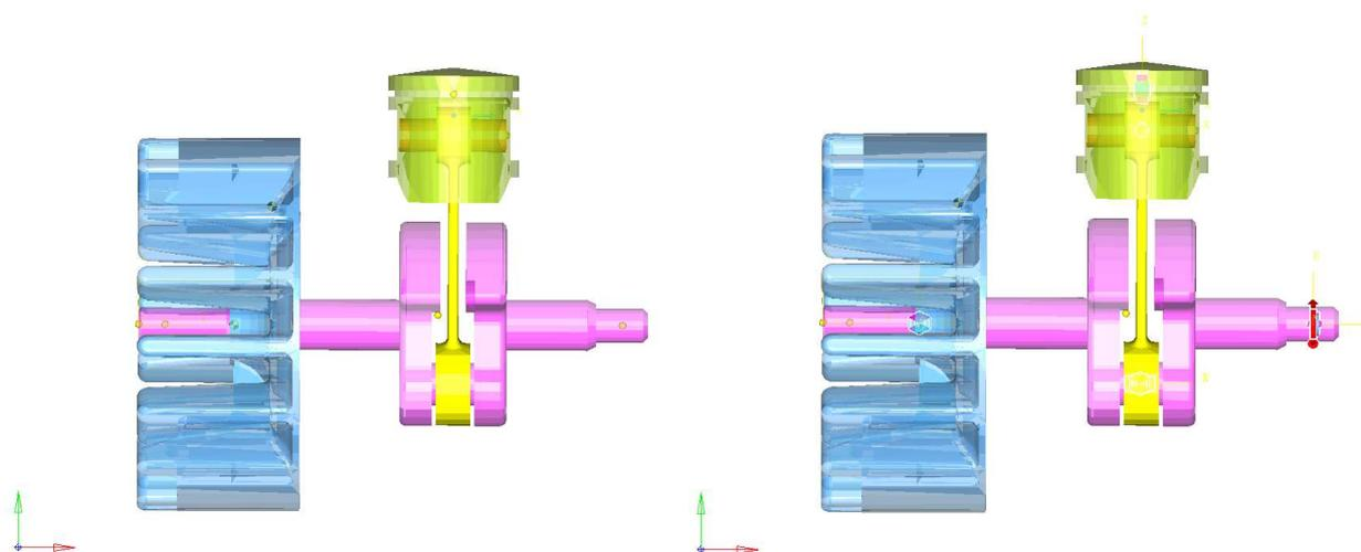
Figure 1: Imported Step Model, Applied Joints Using Motion View
