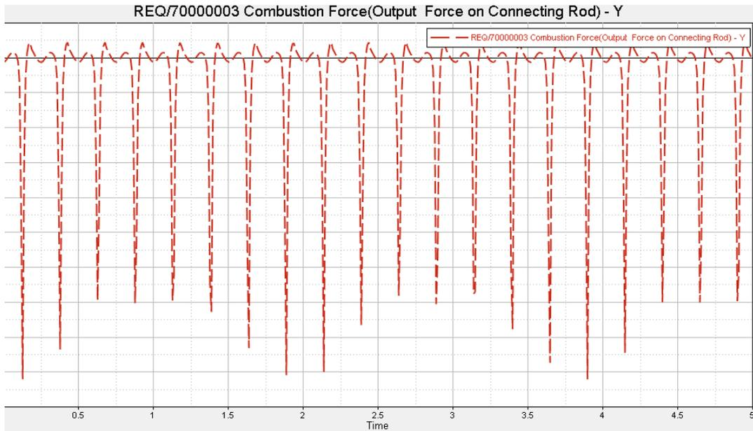
Figure 4: Force on the Connecting Rod
