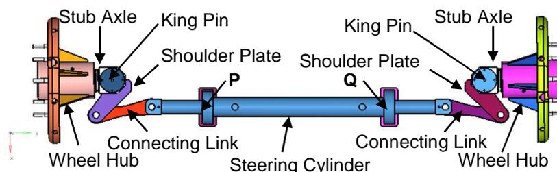
Figure 1: Steering Mechanism
