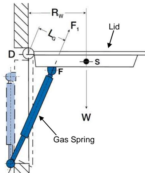
Figure 3: Lid Mechanism [4]
