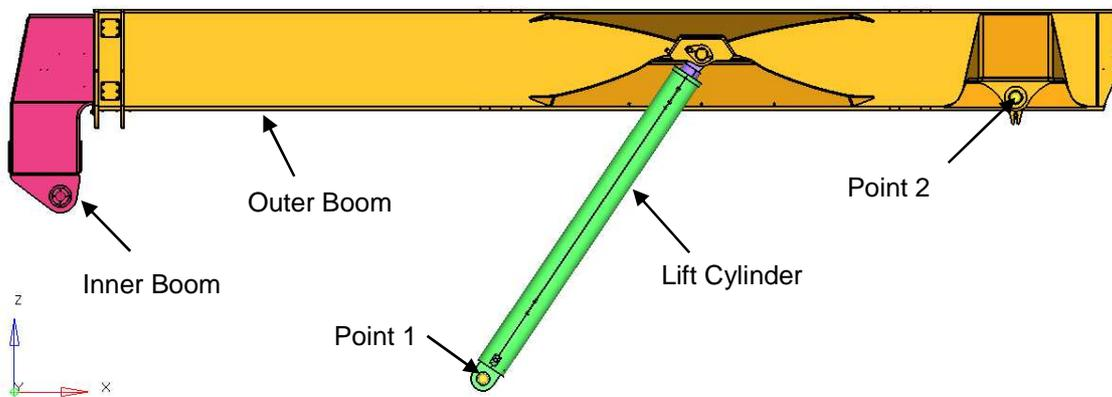
Figure 2: Boom Lifting Mechanism
