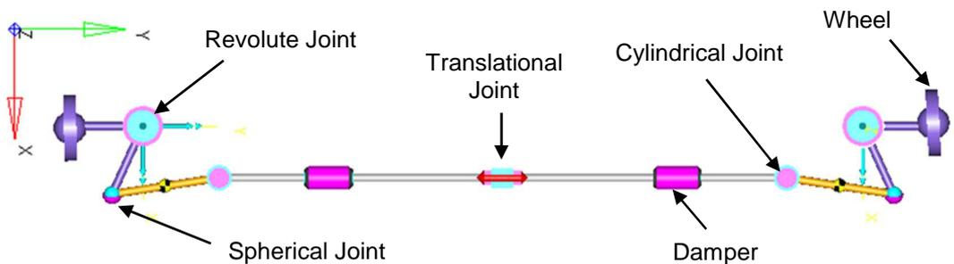
Figure 4: MBD Model Steering Mechanism
