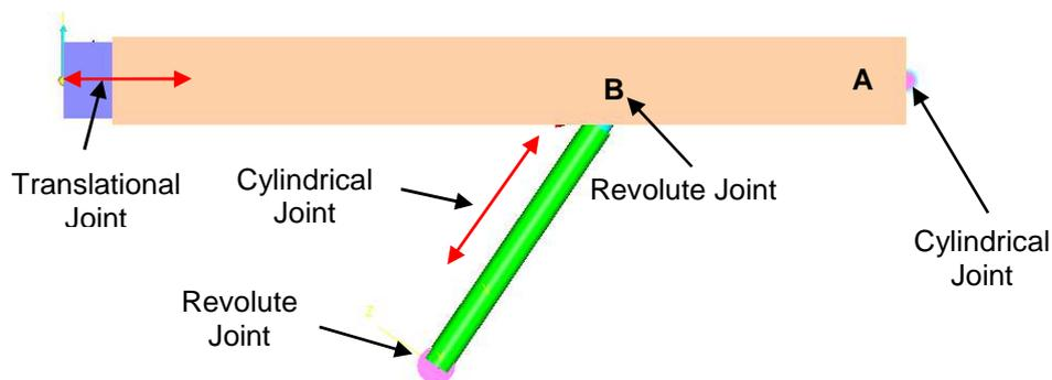
Figure 5: MBD Model Boom Lifting Mechanism
