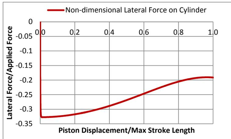
Figure 8: Ratio of Lateral Force to Applied Force on Steering Cylinder
