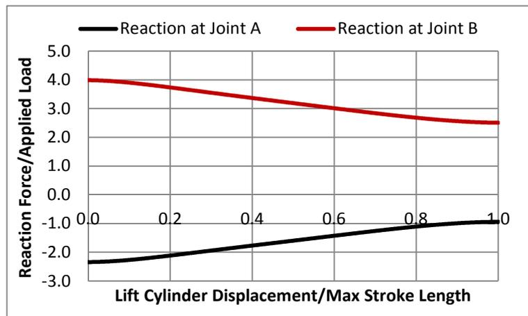
Figure 9: Ratio of Reaction Force to Applied Load on Joints A and B
